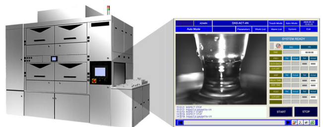
FIGURE 1. The computer vision system embedded in the currently operating semiconductor manufacturing equipment for photo lithography inspection.
