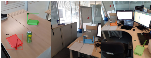
FIGURE 3. Examples of manually annotated images with bounding boxes around USRPs, used for fine-tuning the model pretrained on the COCO dataset.
