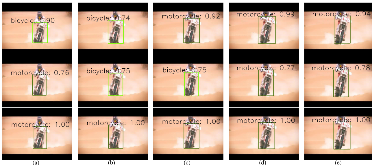
FIGURE 4. The visual examples on ImageNet VID validation sets. (a)–(e) are consecutive frames from one video clips. From top to bottom, three rows shows the detection results of Faster R-CNN, FGFA, BFAN, respectively. These three methods all use ResNet-101 as feature extraction backbone. The dark green boxes labeled “motorcycle” are correct, and the light green boxes labeled “bicycle” are incorrect. The proposed BFAN method outperforms other two object detection methods.
