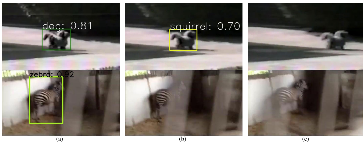
FIGURE 5. Limitation of the proposed BFAN method. (a), (b) and (c) are three frames in serial but not consecutive. The top row shows the failure cases due to the too blurry appearance. The bottom row shows the failure cases due to the occlusion. The frames in the first column both show the correct result, and the frames in the latter two columns all show the failure cases.
