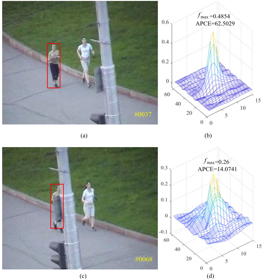
FIGURE 6. Response of frame in the Jogging sequence of OTB2015. (a) Frame #0037. (b) Response of object in frame 37. (c) Frame #0068. (d) Response of object in frame 68. The red bounding boxes indicate the tracking results of the proposed approach with the high-confidence update strategy. When the target is occluded, f_{\max} and APCE decrease obviously, and the template update is not carried out.
