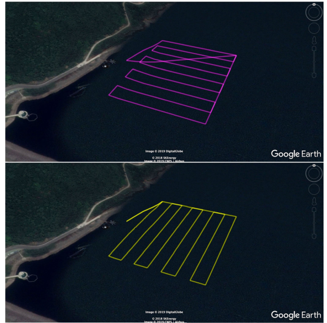
FIGURE 5. Planned USV trajectories for map construction (upper) and GN validation (lower).
