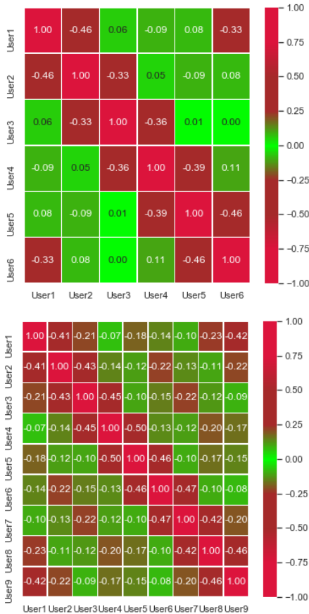
FIGURE 1. Matrix with pair-wise label correlation coefficients for a system with K = 6 (top) and K = 9 (bottom) users sorted according to increasing angles-of-arrival ( N_{BS} = 4 antennas).
