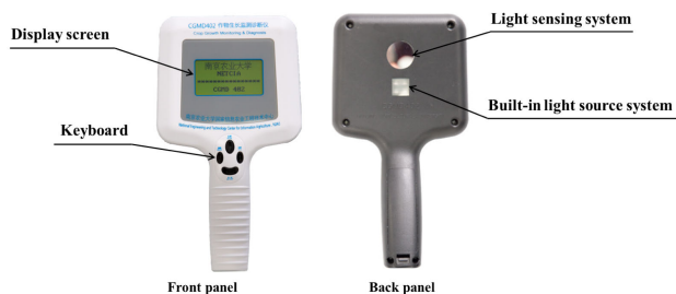
FIGURE 3. The overall structure of the CGMD apparatus.
