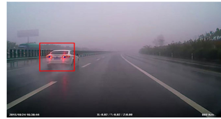
FIGURE 5. The final effect of identifying the vehicle through taillight segmentation.
