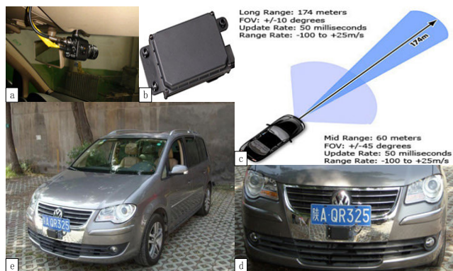
FIGURE 8. Experimental equipment. (a) Camera installation position. (b) mm-W radar. (c) mm-W radar measurement range. (d) mm-W radar installation position. (e) TOURAN car.
