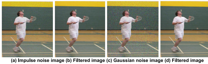
FIGURE 5. Denoising effect diagram of adaptive median filter.
