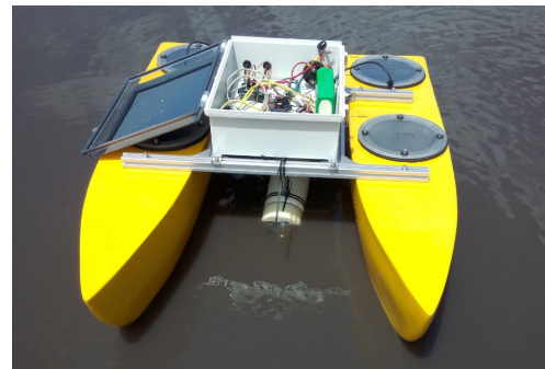
FIGURE 2. Prototype of ASV designed for the exploration of Ypacaraí Lake in [1].
