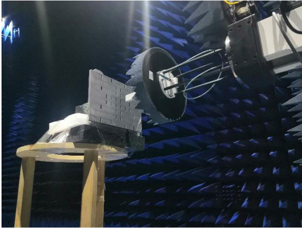
FIGURE 12. Photograph of the near-field measurement environment.
