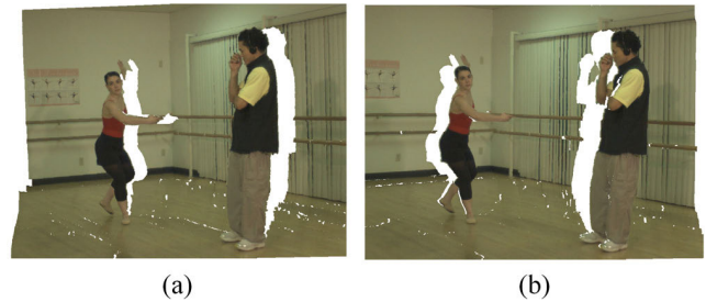
FIGURE 4. Synthesized result of modified 3D warping. (a) Right synthesized virtual image. (b) Left synthesized virtual image.
