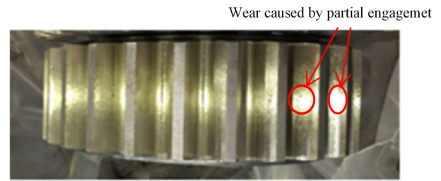
FIGURE 20. The partial meshing at Z3 gear because of tooth shape and tooth direction error.
