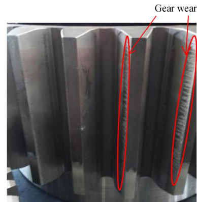
FIGURE 13. The abrasion fault at Z18 gear.
