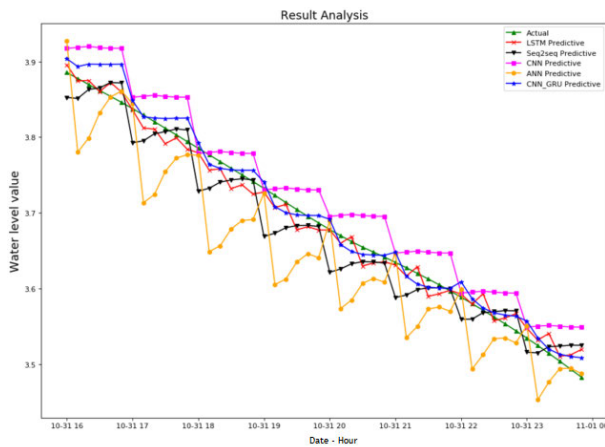
FIGURE 11. The water level predicted by LSTM/Seq2seq/CNN/ANN/Conv-GRU at Chang'an Bridge station.
