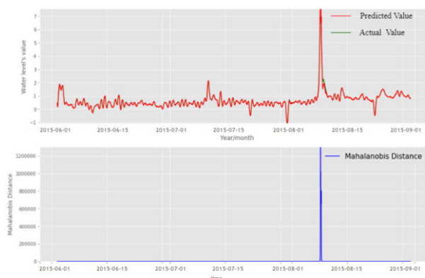
FIGURE 23. Upper: The prediction by Conv-GRU (red) and the actual water level value (green) at Zhongzheng Bridge in 2015; lower: the Mahalanobis distance.
