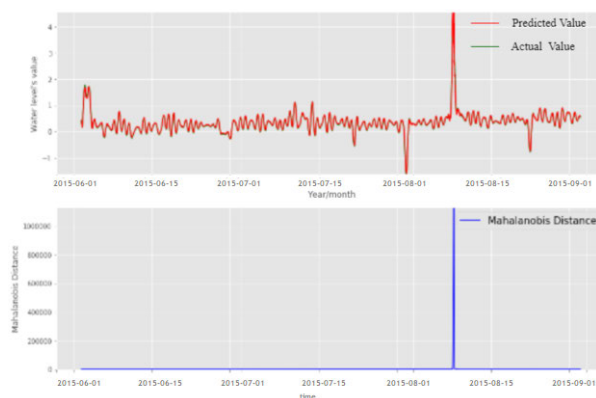
FIGURE 26. Upper: The prediction by Conv-GRU (red) and the actual water level value (green) at Taipei Bridge in 2015; lower: the Mahalanobis distance.
