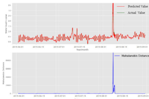
FIGURE 25. Upper: The prediction by Conv-GRU (red) and the actual water level value (green) at Zhongshan Bridge in 2015; lower: the Mahalanobis distance.
