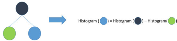
FIGURE 6. Histogram accelerating. (Note: the feature number of the right leaf node is equal to the feature number of the root node minus the feature number of the left leaf node).
