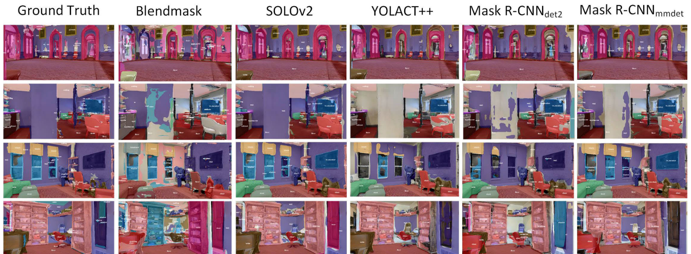
FIGURE 5. Examples of instance segmentation using different neural network models on images from HISNav-test dataset.
