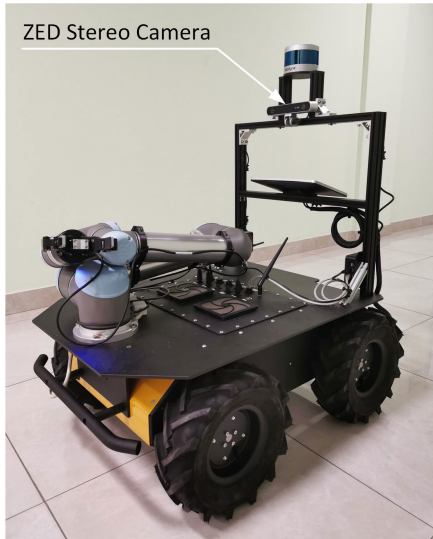
FIGURE 4. Ground robot platform based on Clearpath Husky chassis with ZED camera. It was used for experiments with proposed algorithms.
