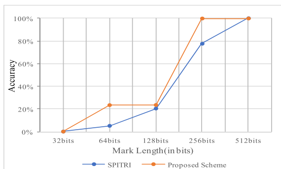
FIGURE 15. Comparison of accuracy between Vijayalakshmi’s method and method proposed in the present study in a network environment without IXP services.
