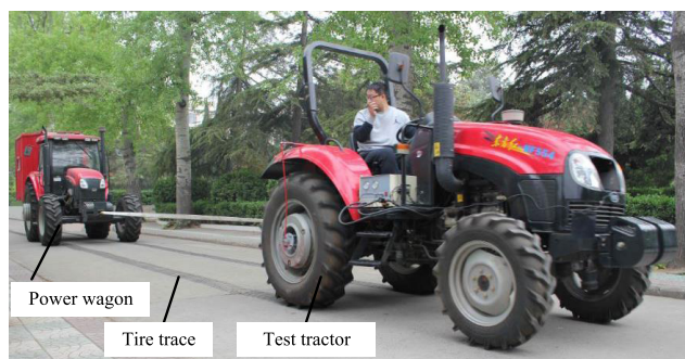
FIGURE 9. Tractive characteristic test of the tractor.
