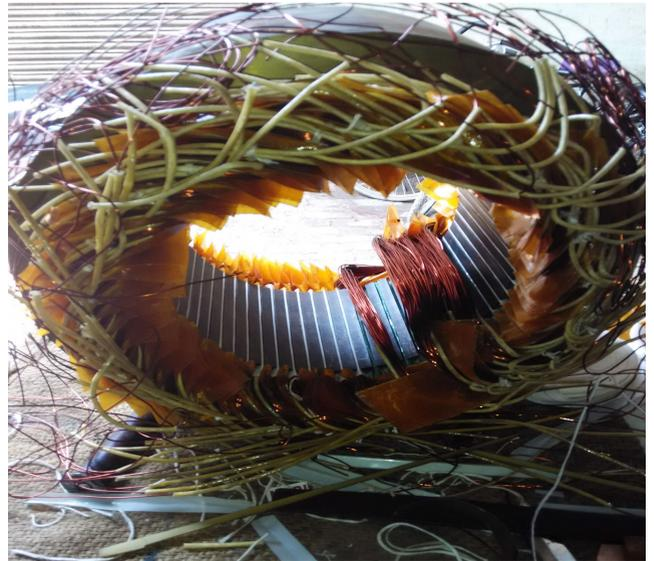
FIGURE 14. Stator winding intermediate process.
