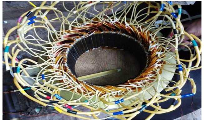
FIGURE 15. Stator with complete winding.
