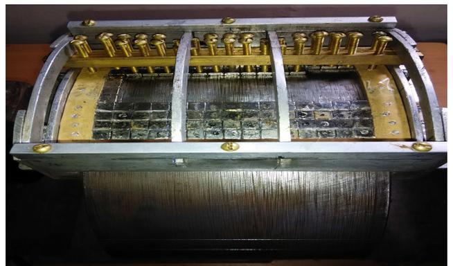
FIGURE 16. Magnet Pasting Process.
