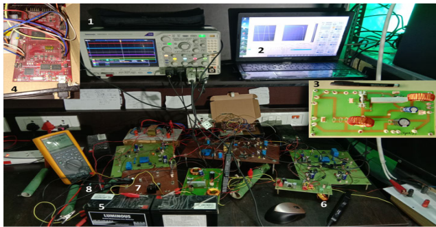
FIGURE 11. Experimental prototype of DC-NG: 1. DSO, 2. TerraSAS ETS80, 3. FBDC, 4. Digital Controller, 5. Battery, 6. Source converter, 7. Load converter, 8. Driver and Sensor Circuits.
