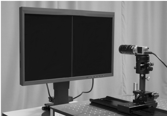
FIGURE 17. Prototype display MTF measurement system.
