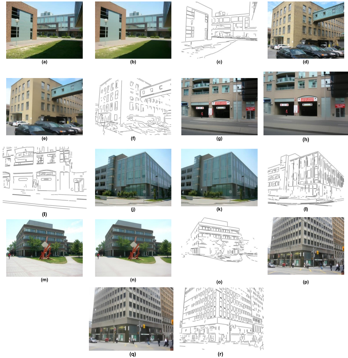
FIGURE 5. Structural features of building facades extracted through the proposed method. (a), (d), (g), (j), (m), and (p) are the original facade images. (b), (e), (h), (k), (n), and (q) are the texture fused images through RTV. (c), (f), (i), (l), (o), and (r) are the structural features of building facades extracted through the proposed method.
