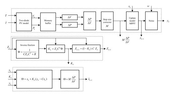
FIGURE 4. Block diagram of Kalman-MPPT architecture.
