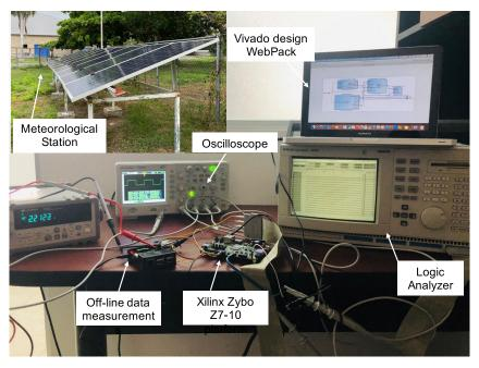
FIGURE 12. HW/SW codesign with the Kalman-MPPT as the coprocessor PL unit.
