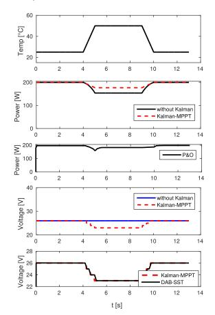
**FIGURE 14.** Results of Kalman-MPPT implementation for temperature variations.
