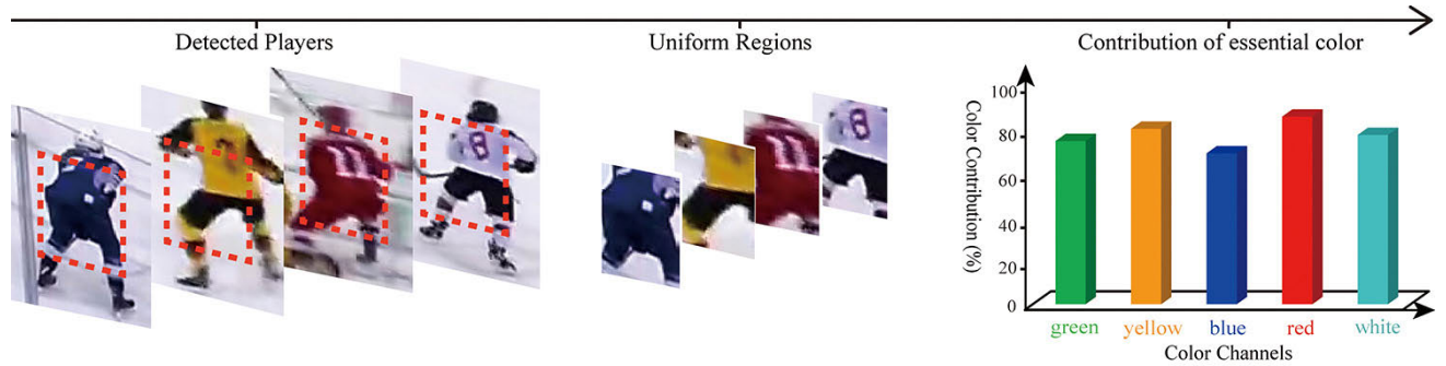
FIGURE 2. Procedure of team classification. The uniform regions were cropped from the detected players that contained discriminate color feature of uniforms, from which the contribution of essential color were extracted to determine the team affiliations.
