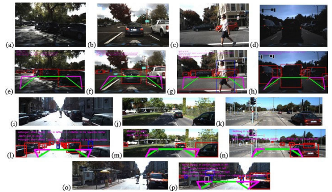
FIGURE 24. Input Udacity [66]/KITTI [24] dataset images and their respective outputs along with corresponding proximity alerts and navigation suggestions. (a), (b), (c), (d), (i), (j), (k), (o) are KITTI/Udacity dataset inputs fed to the AMMDAS. Adaptive left, center, right-FOV markings are drawn along with bounding boxes around detected objects, simultaneously the AMMDAS’s final output proximity alerts and corresponding navigation suggestions are inscribed on these marked input panoramic images to simulate the final DAS output illustrations (e), (f), (g), (h), (l), (m), (n), (p). (a), (b), (c), (d) inputs belong to the Udacity road dataset; and (i), (j), (k), (o) belong to the KITTI dataset. Detailed description on the generated outputs is given in Table 5.
