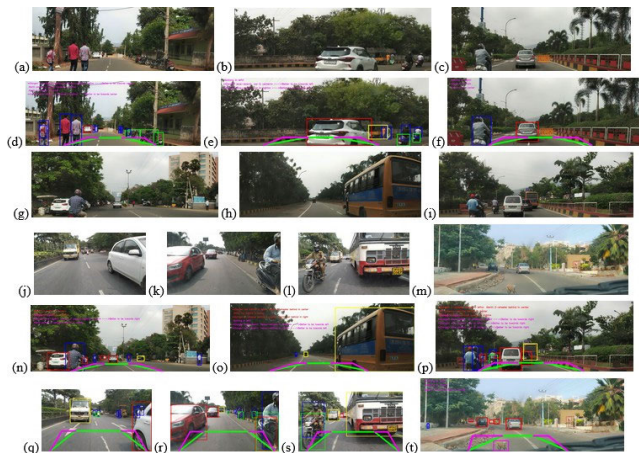
FIGURE 22. (a)-(t) consists of sample input panoramic images along with corresponding outputs which consists of framed proximity alerts and navigation suggestions. (a), (b), (c), (g), (h), (i), (m) are front view's panoramic input fed to the AMMDAS, simultaneously with (j), (k), (l) rear view's input feed. Here (g, j), (h, k), (i, l) pairs belongs to the same respective input instances. Adaptive left, center, right-FOV markings are drawn along with bounding boxes around the detected objects, and the AMMDAS's final output proximity alerts and corresponding navigation suggestions are also inscribed on these marked input panoramic images to simulate the final DAS output illustrations ((d), (e), (f), (n), (o), (p), (t)). Detailed description on the generated outputs is given in Table 4.
