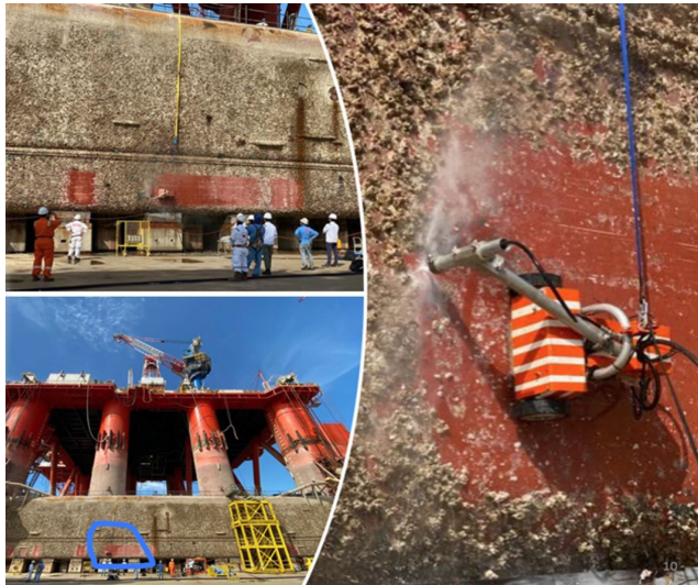
FIGURE 1. ShipHull surface with corrosion and blasting by Hornbil.
