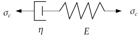
FIGURE 1. Maxwell rheological model ( \sigma_c defines the external load which is regarded as constant; E and \eta represent the elastic modulus and the viscosity coefficient, respectively).
