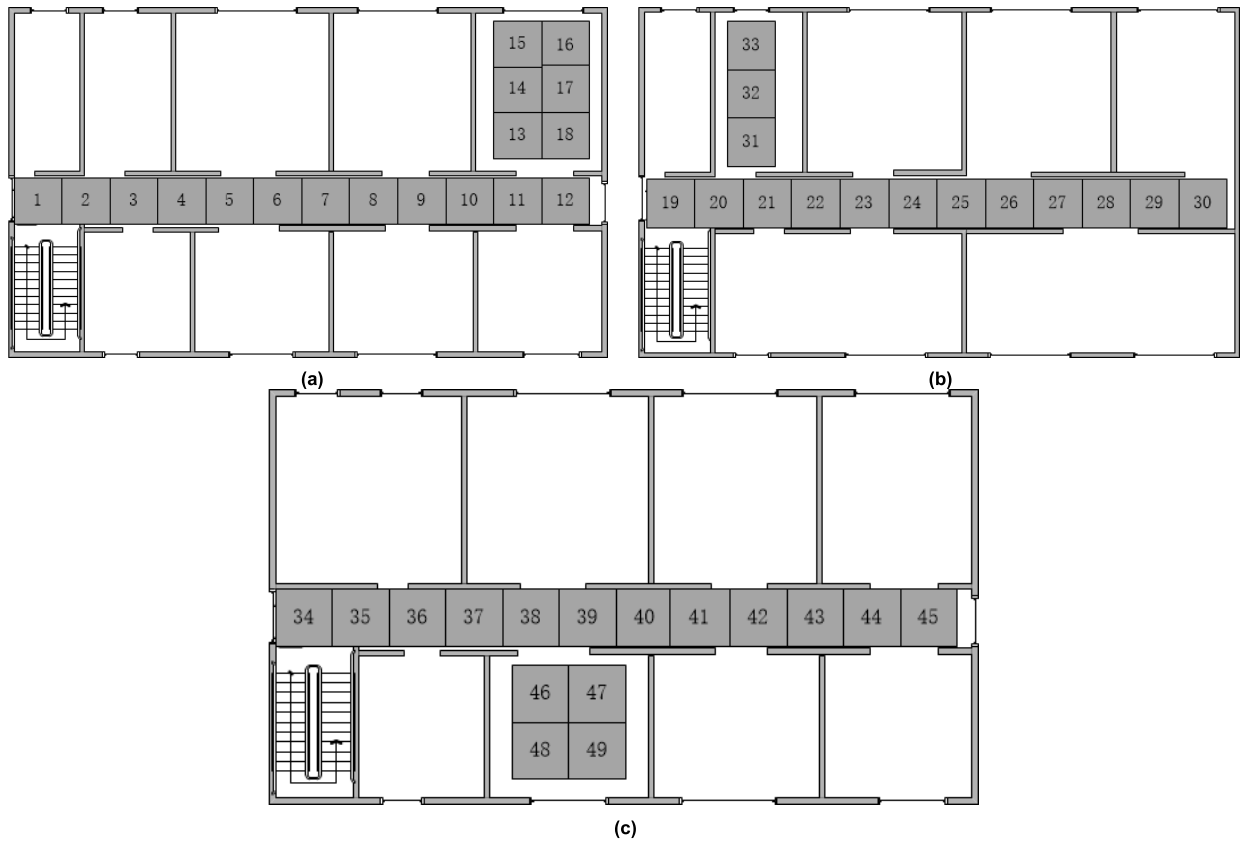
FIGURE 8. Location of the 49 reference points (1.8 m × 1.8 m each, with magnetic field data collected at the four corners of each region).
