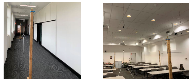
FIGURE 15. Setup of the two tests. For the 2D test (bottom left), two base stations were located at (x_1, y_1) and (x_2, y_2) , and the mobile station was located at (x, 0) , x=0, 2, 4, 6, 10 and 15m . For the 3D test, one more base station was located at (x_3, y_3) as using TOA measurements only for 3D positioning requires at least three base stations, and the mobile station was located at (0, 0, z) where z=0.18, 1.38 and 2.23m .
