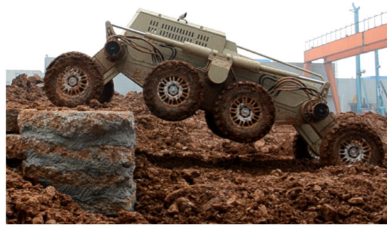
(b) Obstacle surmounting of the ATV
