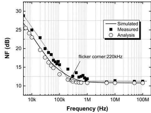
**FIGURE 14.** NF with respect to the IF frequency,  $f_{IF}$ .
