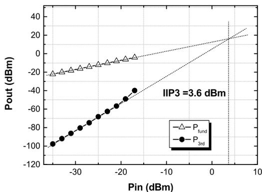
**FIGURE 16.** IIP3 results at 1 GHz frequency point.
