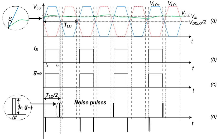
**FIGURE 2.** (a) Differential trapezoid periodic LO stimulus applied at the switch stage. The mixer output response with respect to LO stimulus decomposed into (b) noiseless switched bias current, (c) noiseless switched transconductance, and (d) noise pulses.
