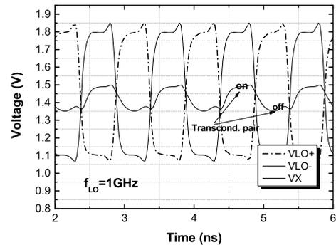
**FIGURE 15.** Steady-state time-domain response at the tail net.
