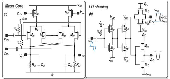
FIGURE 11. (a) Proposed mixer core and (b) LO generation chain.
