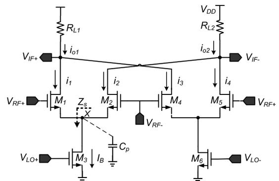
FIGURE 1. Diagram of the improved switched transconductor mixer.
