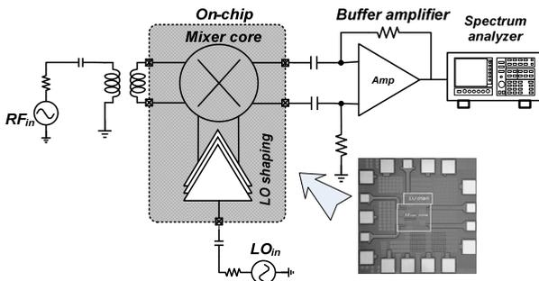
**FIGURE 12.** Test setup and micrograph of the proposed mixer.
