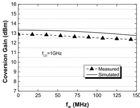
**FIGURE 13.** Conversion gain with respect to IF when LO frequency,  $f_{LO}$  is fixed at 1 GHz.
