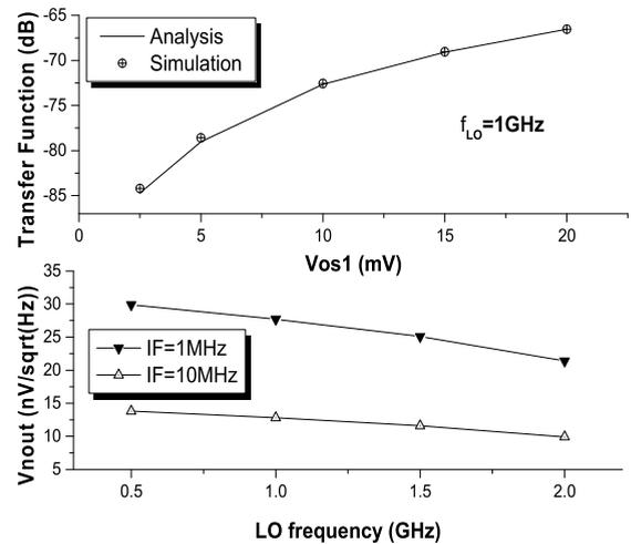
**FIGURE 9.** Transfer function of the switch flicker noise to the output current noise at the output of the mixer due to mismatch represented by offset voltage,  $V_{os1}$ . (b). Output noise with variations of LO frequency for the mixer.
