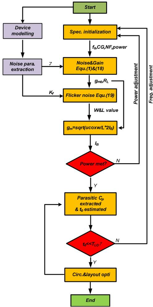
FIGURE 10. Design flow of the proposed mixer.
