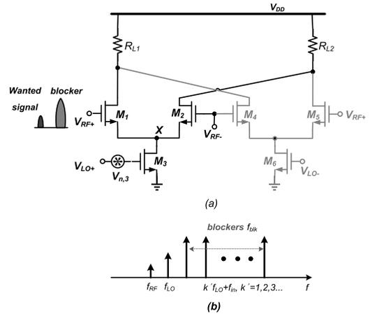
FIGURE 4. (a) Diagram for switch flicker noise transfer mechanism analysis due to (b) blockers coexistence with the wanted signal at RF port.
