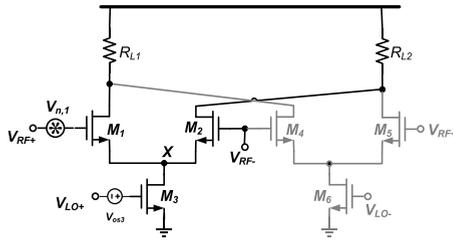
FIGURE 3. Diagram for transconductance flicker noise transfer mechanism analysis.
