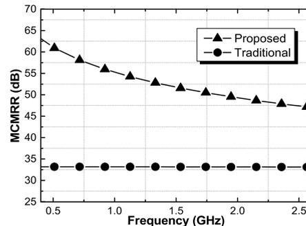
FIGURE 7. Calculated mixer common-mode rejection ratio (MCMRR).
