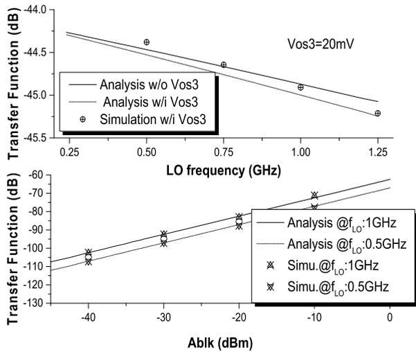
**FIGURE 8.** Transfer function of the transconductance flicker noise to the output current. (b). Transfer function of the switch flicker noise to the output current in the presence of the blocker with  $f_{blk} = f_{LO} + f_{in}$ .
