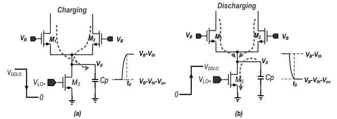
FIGURE 6. Diagram of parasitic capacitance CP (a) charging and (b) discharging at tail net.
