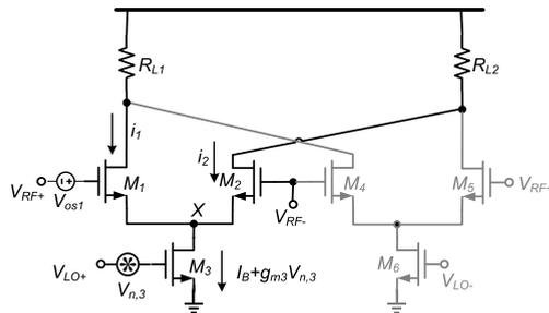
FIGURE 5. Diagram for switch flicker noise transfer mechanism analysis due to mismatch.
