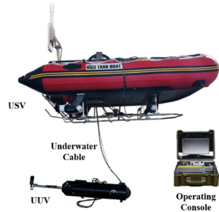
FIGURE 2. Unmanned Marine Vehicle (UMV) System configuration.
