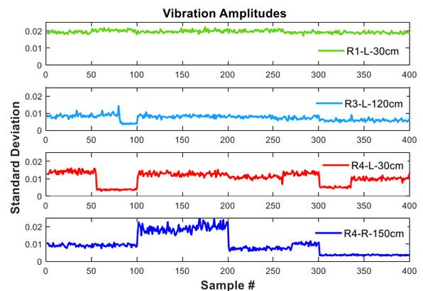
**FIGURE 9.** Standard deviation of vibration amplitudes versus number of samples, for the locations R1-L-30cm, R3-L-120cm, R4-L-30cm, and R4-R-150cm due to leak at R4-R-15cm. This is used as training data for the two SVM models. For each leak condition 100 Sample values are used. As shown on x-axes, first 100 Sample values are for no leak condition, next 100 for small leak and then for medium leak and large leak conditions, respectively.
