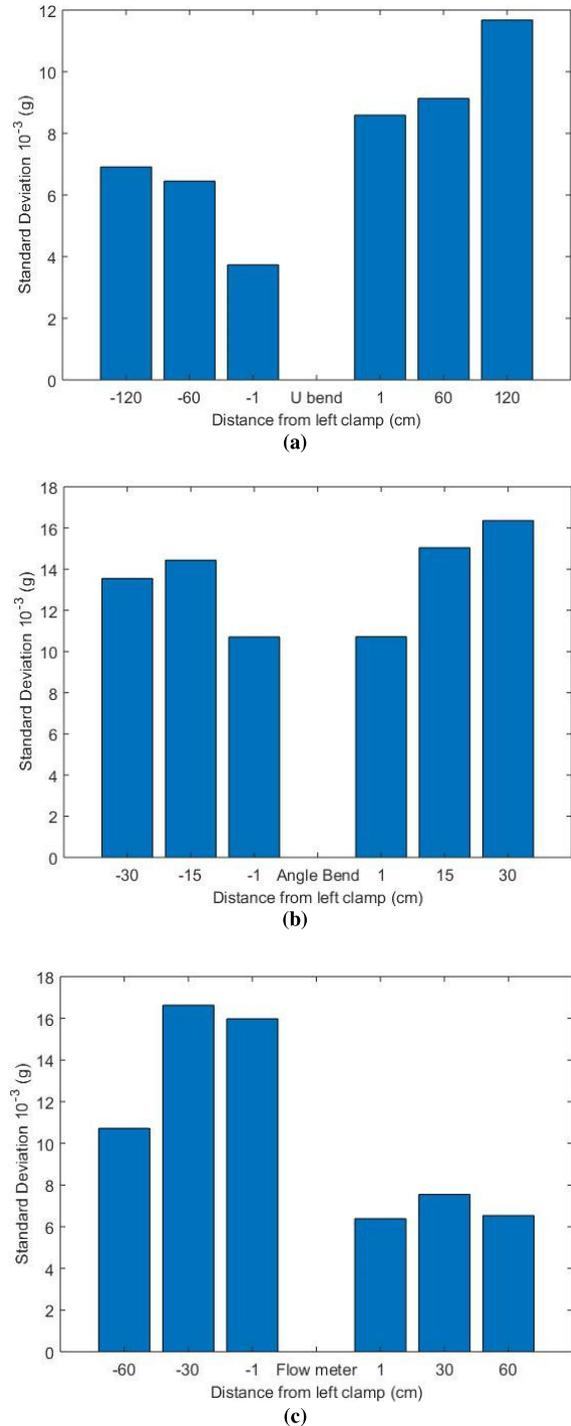
**FIGURE 6.** Standard deviations of vibrations signals with respect to distance, (a) before and after U-bend between sections R2-L and R3-L, (b) before and after the angled bend in sections R1-L and R4-L, and (c) before and after the flowmeter in section R1-L. Negative and positive distances on the x-axis respectively show distances on left and right sides from angle bend / flow meter.
