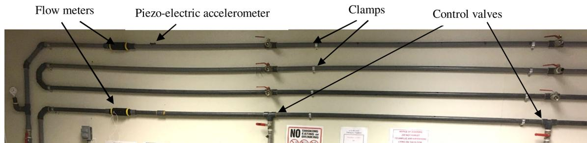
**FIGURE 1.** Actual wall mounted setup.
