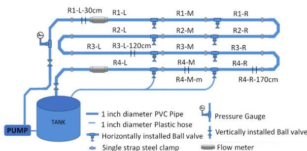
**FIGURE 3.** Layout showing labels of pipeline sections, and examples of some locations in which distance is measured with respect to the clamp on the left-hand side (diagram not drawn with scale).
