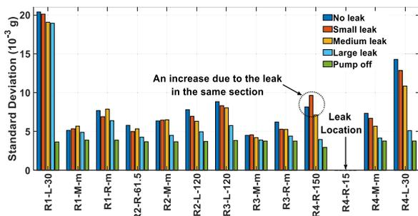
**FIGURE 8.** Standard deviation at different locations in all pipe sections under different leak conditions and in an order given by the direction of flow.
