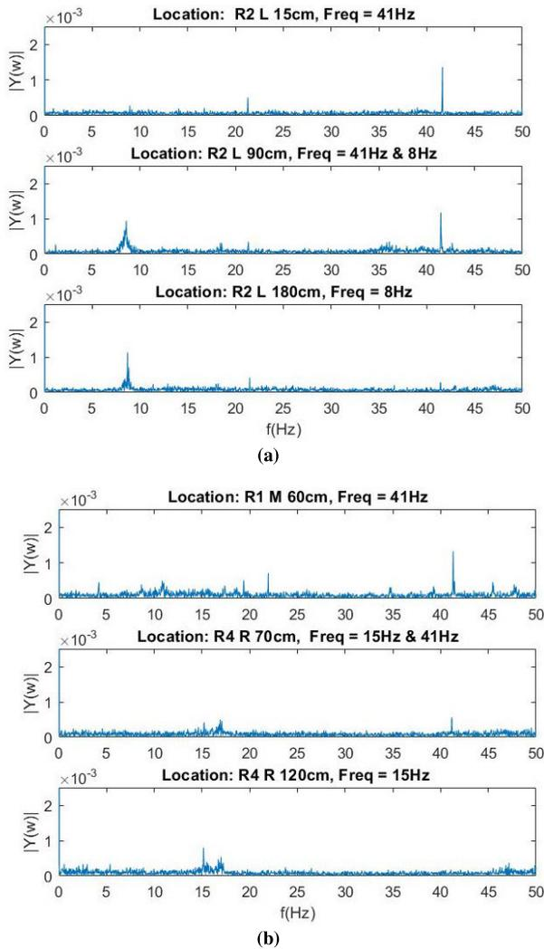
**FIGURE 5.** Vibration frequency analysis. (a) three locations in sections R2-L. (b) Three locations in sections R1-M and R4-R.
