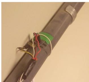
**FIGURE 2.** Accelerometer ADXL-345 used on pipeline with its mounting setup facing upwards.
