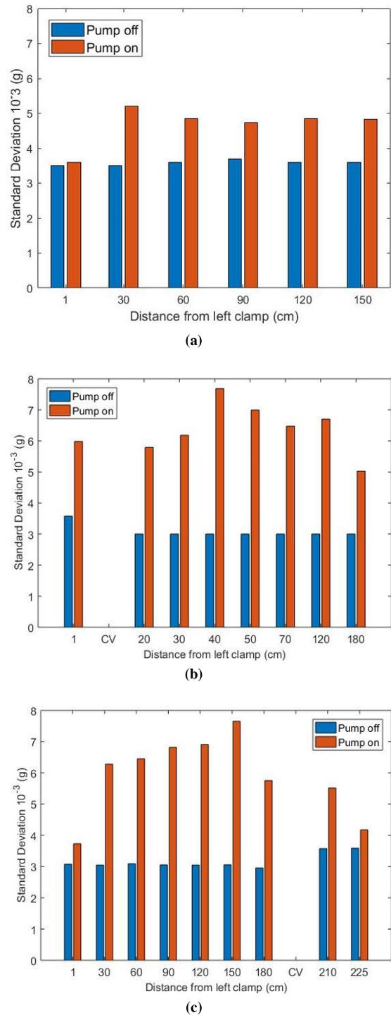
**FIGURE 4. Standard deviations of vibrations at (a) five locations in section R1-M, (b) seven locations in section R4-R, and (c) eight locations in section R2-L.**
