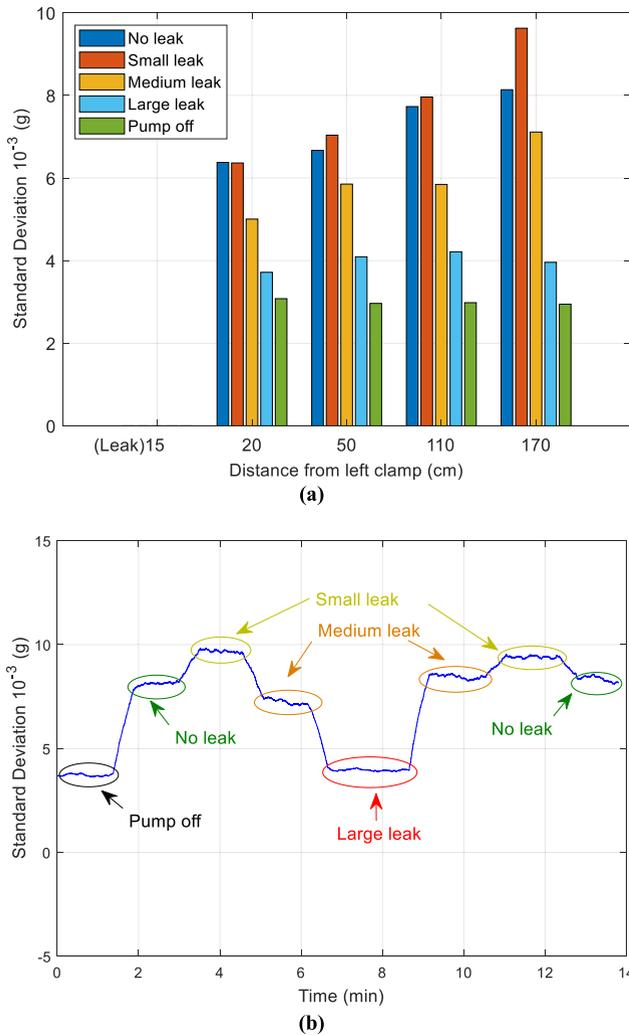
**FIGURE 7.** Standard deviation (SD) of vibrations at 4 locations on R4-R for various conditions, (b) A full cycle showing SD of vibrations under the 4 leak conditions in section R4-R-150cm.
