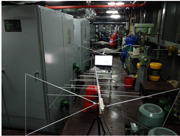
FIGURE 9. Measurement of the EMR signals from four generators that were operated at their rated condition.
