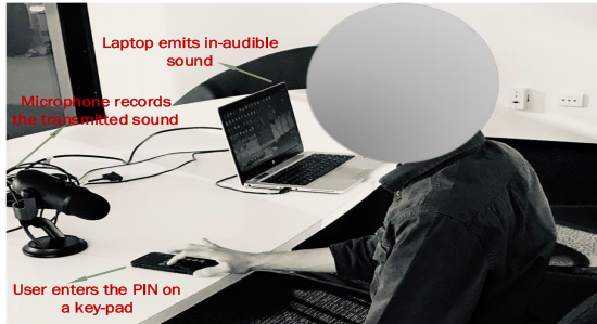
FIGURE 22. Evaluation setup of E-ID.
