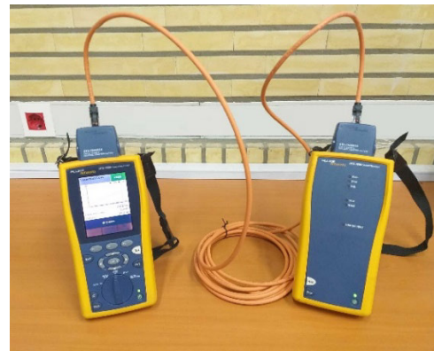
FIGURE 9. Typical twisted pair cable testing with Fluke DTX-1800 cable analyzer.
