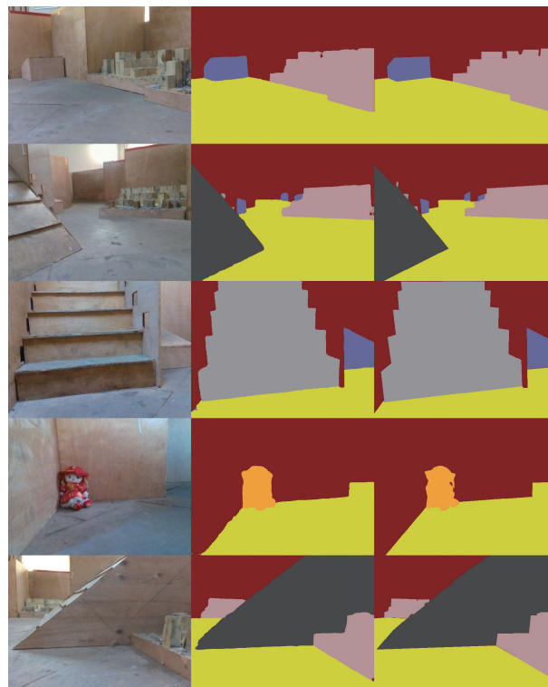
FIGURE 7. Example results of segmentation test. Left: RGB images, middle: segmentation result, right: ground truth.
