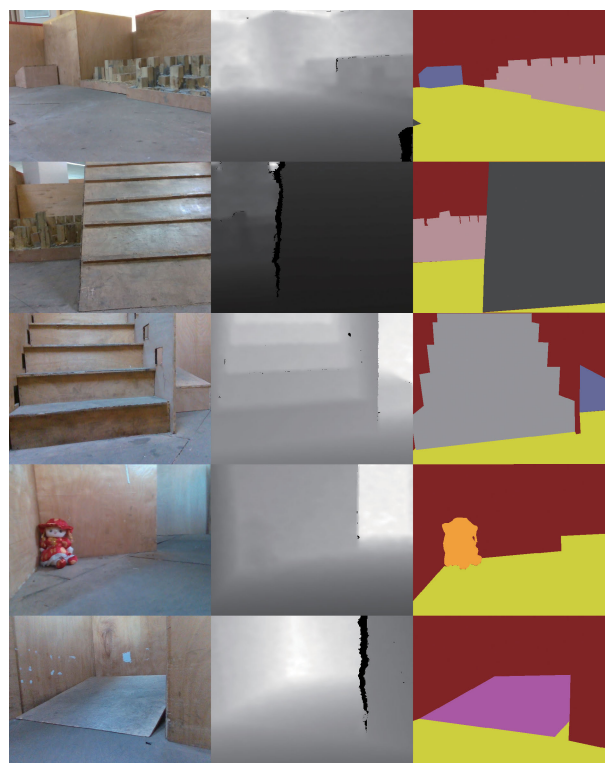
FIGURE 4. Dataset of the RRL competition environment. Left: RGB images, middle: depth images, right: semantic labels.
