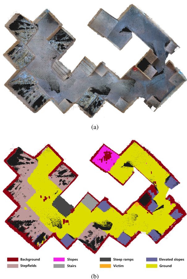
FIGURE 1. Example dense semantic map generated by our approach. (a) Colored point-cloud map of an RRL test field (view from above). (b) Corresponding semantic map including eight types of terrain.
