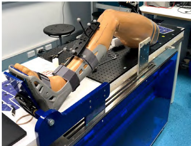
FIGURE 2. Leg Manipulator robot developed for leg surgery (Patent No. 2019900476). The position of the foot determines the pose of the knee and hip joints. The robot model of the leg provides the coordinates of the foot to the robot, and using the robot's inverse kinematic model the foot can be placed into that position.
