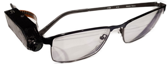
FIGURE 4. AIM-2, an egocentric wearable camera with food intake detection sensors.
