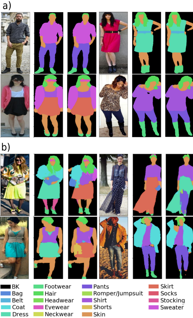
FIGURE 7. Segmentation results on the test set based on: a) highest and b) lowest IOU score. This Figure shows the input image, ground truth, and the predicted class from left to right, respectively.
