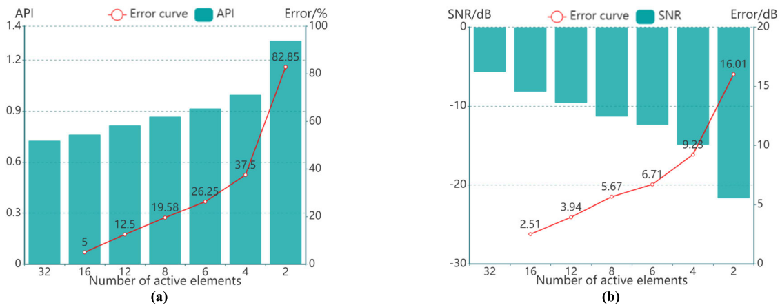
FIGURE 11. Comparison of API and SNR of TFM images with different sparse arrays. (a) API; (b) SNR.
