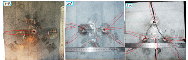
FIGURE 20. Fragmentation in the back surface of specimen 3.
