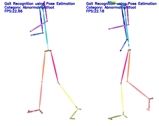
FIGURE 16. Output result of the CNN-based classifier with respect to Fig.8, and Fig. 12 with detected category as Abnormal Right Foot.
