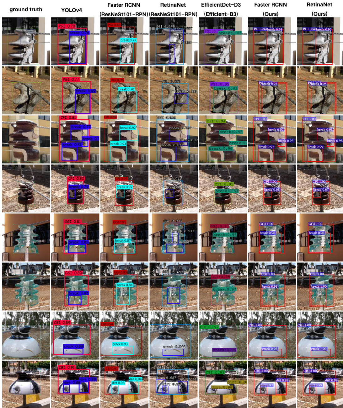
FIGURE 4. Performance of EfficientDet-D3 (EfficientNet-B3), RetinaNet (ResNeSt101-RPN), Faster RCNN (ResNeSt101-RPN), YOLOv4 (CSPDarknet-53), Faster RCNN (Ours) and RetinaNet (Ours). The first column is the insulator type, insulator position, defect category and defect location labelled by LabelImg. The text above the rectangle indicates the insulator type or defect type detected by the network. The following number indicates the accuracy of the object detected by the network.
