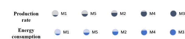
FIGURE 19. Ranking for non-homogeneous line with non-identical machines and buffers and \lambda_j = \lambda and \mu_j = \mu .
