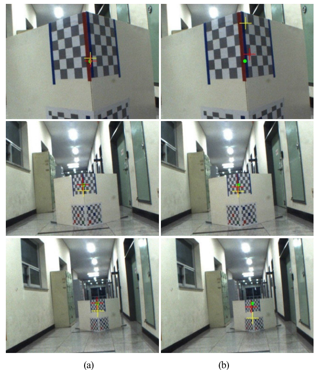
FIGURE 10. Comparison of projection error on a dummy camera (green circle: ground truth, yellow cross: by the Hu [12] algorithm, red cross: by the proposed algorithm, first row: 1m, second row: 3m, third row: 5m) (a) by result of T2 in Table 5 (b) by result of T9 in Table 5.
