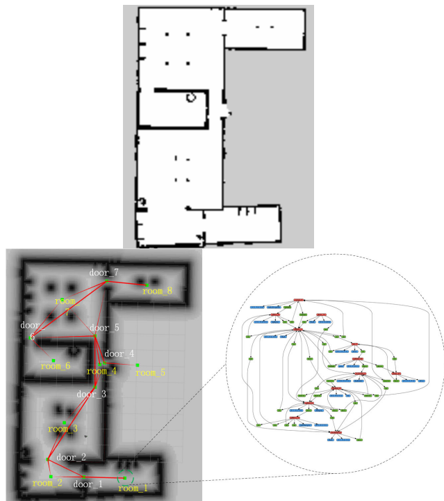
FIGURE 4. Constructed map: (a) The metric map, above the figure, is built with the collected 2D laser scan in the form of an occupancy grid map. (b) The topological map, below the figure, is constructed with manual assistance, nodes and edges are attached with semantic information. Each room node has a scene graph.
