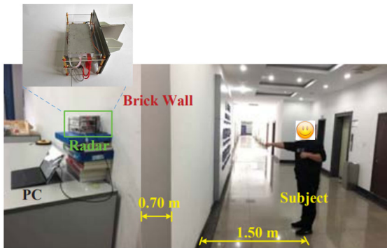
FIGURE 7. The experimental scenario for dataset acquisition with a self-developed TWR.
