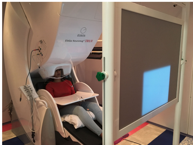
FIGURE 1. The MEG unit (Neuromag; MEGIN, LCC) with a subject. The MEG was kept at upright position with the subject sitting comfortably with their head inside the dewar (sensor cap). The screen was placed at about 90 cm distance from the subject which displayed the stimuli.
