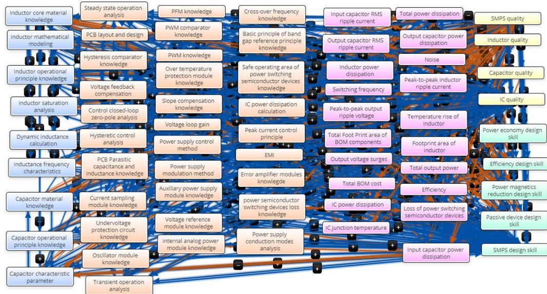
FIGURE 7. An FCM-based SMPS design assistant system.
